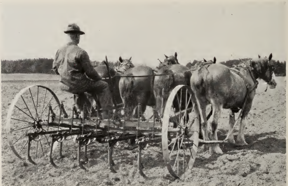
With a four-horse cultivator, one man will average 12.7 acres per day at a cost of 49 cents per acre. The four-horse machine is three feet wider than the one shown above.
