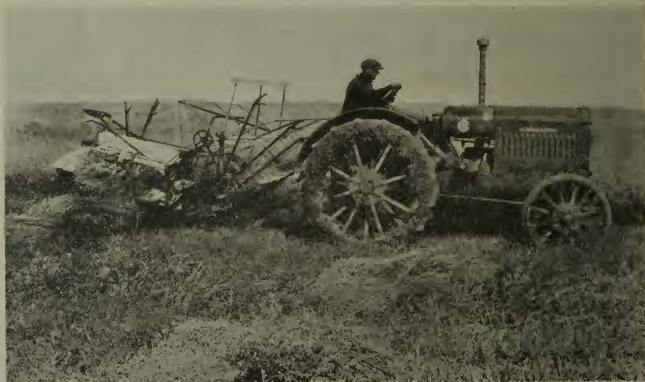
The 4-horse team on an 8-foot binder cuts approximately 18 acres per ten-hour day while the power binder cuts 32 acres. The total costs per acre, however, are practically equal, being $1.05 and $1.07 per acre respectively.
