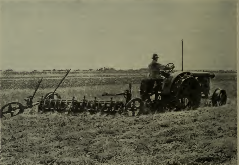
The one-way disc plough can be used to speed up stubble and summer-fallow operations. A nine-foot one-way disc will cover three acres per hour.
