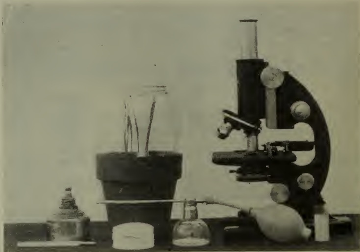
FIG. 10.—Apparatus employed in the isolation of single urediniospores.
