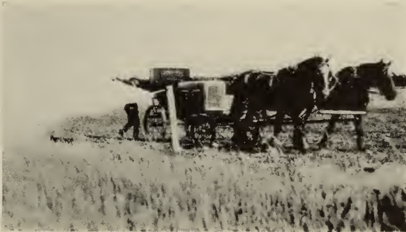
FIG. 25.—Shunck horse-drawn power duster in operation. The dust is discharged through a wide delivery tube at the side.
