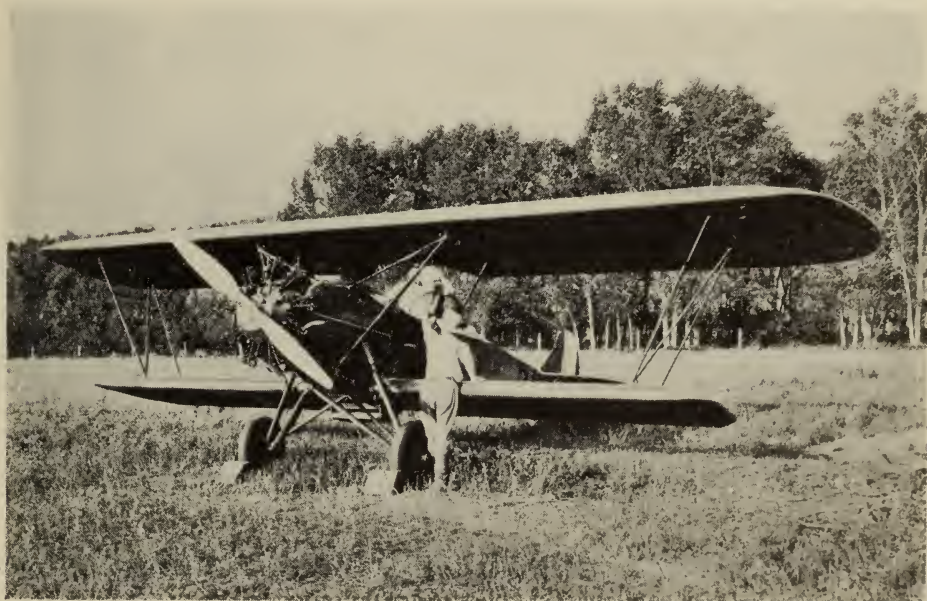
FIG. 27.—Dusting plane (Keystone Puffer) used for aeroplane dusting experiments in Manitoba. Loading the machine with sulphur dust. Hopper capacity 600 pounds.
