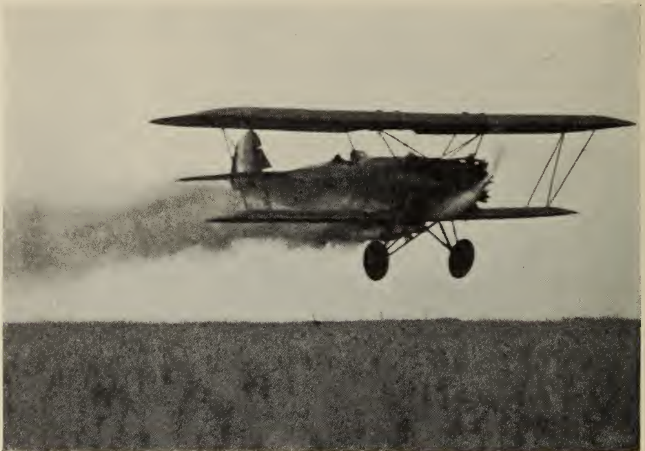
FIG. 30.—Dusting plane in operation showing behaviour of dust after being discharged from hopper. The machine is flying at an altitude of from 10 to 15 feet.
