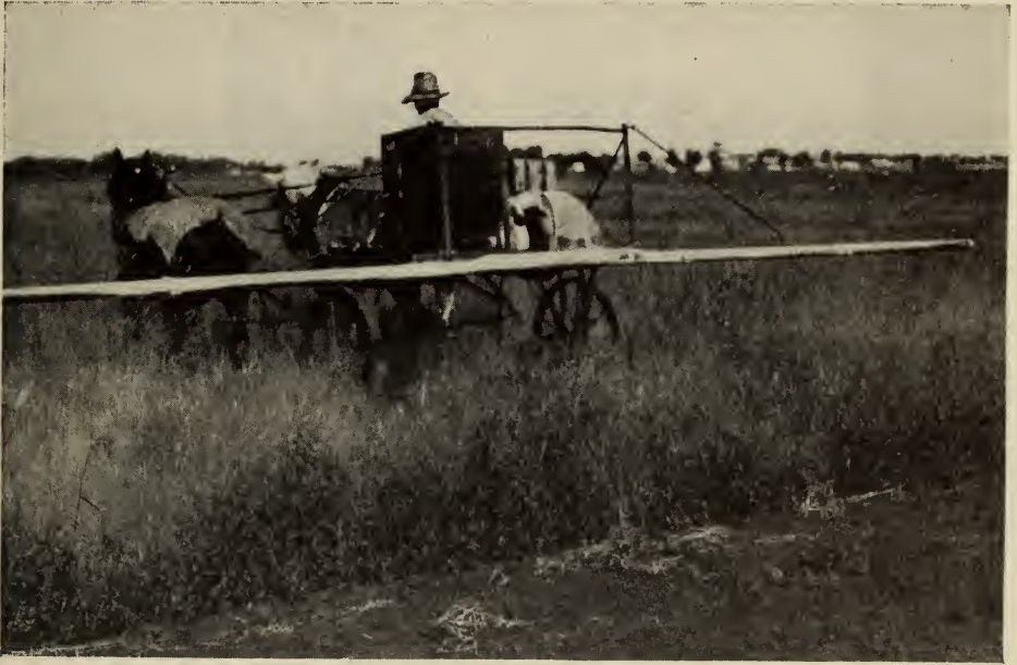
FIG. 26.—Niagara horse-drawn power duster with boom dust distributor. Width of boom 30 feet.
