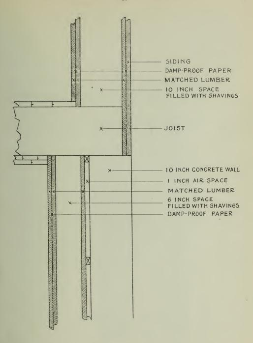
Fig. 2 - Section of Wall at Ceiling of Basement.
