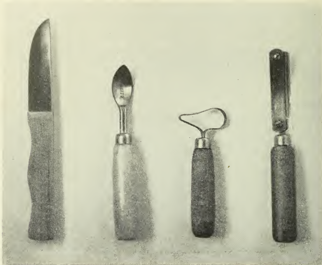
FIG. 5.—Preparation utensils. (Left to right). Cannery knife, peach pitting spoon, pear coring loop, and pear paring knife.
