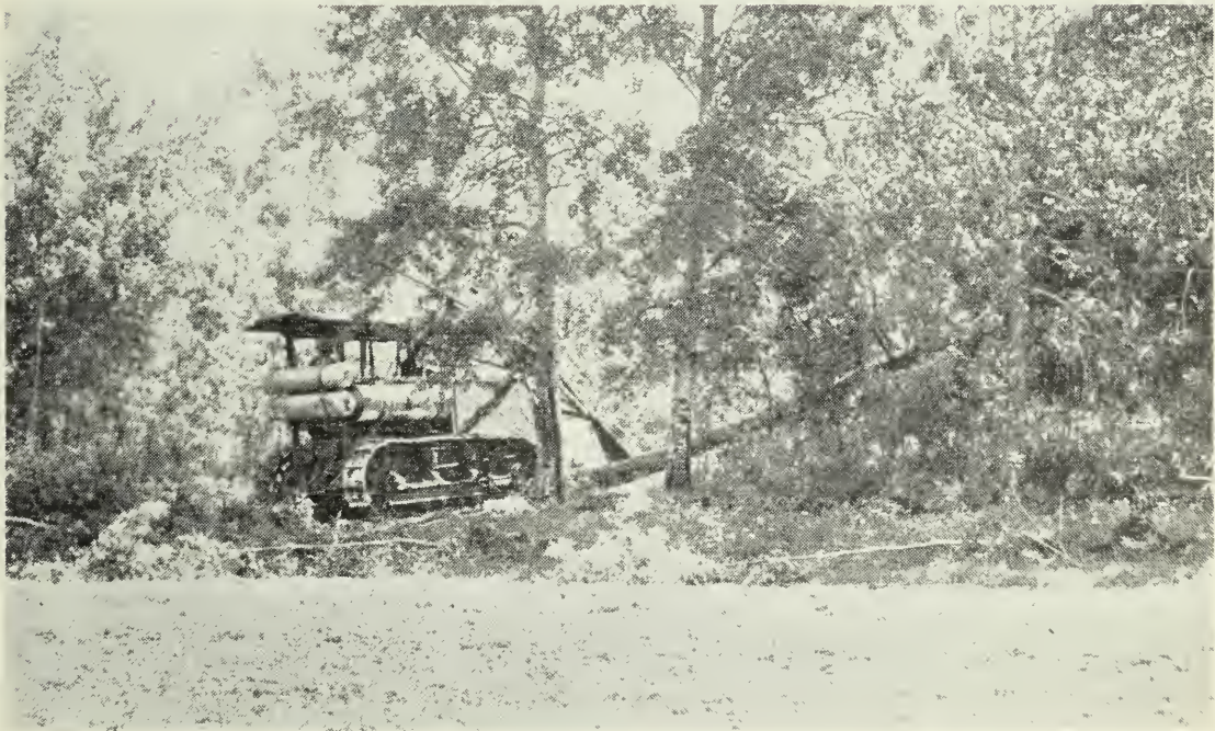
FIG. 2.—A large poplar is sheared off by a crawler tractor brush cutter.
