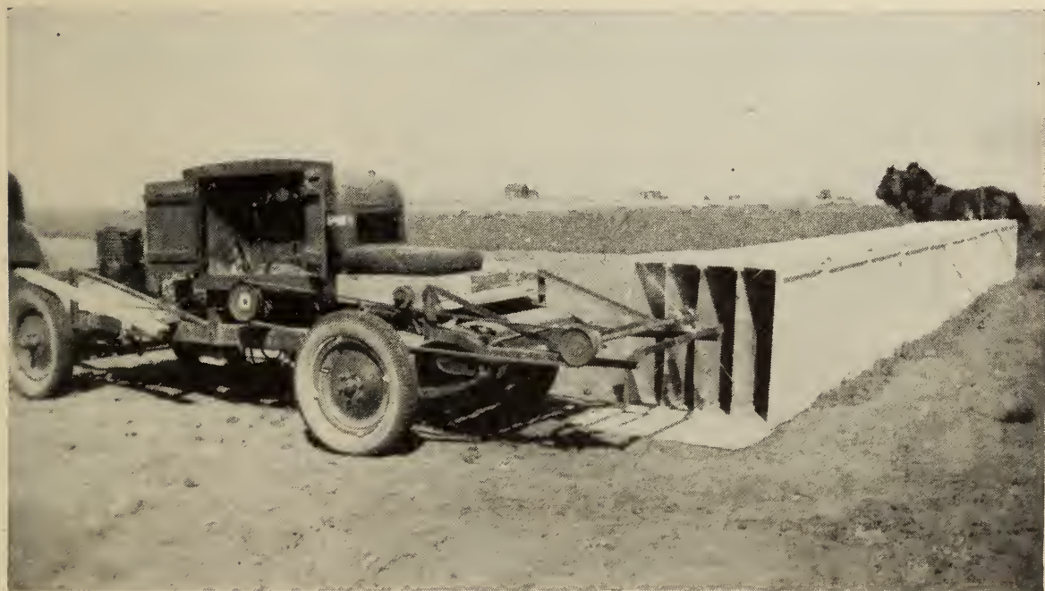
Wind tunnels are used to study soil drifting at the Soil Research Laboratory, Dominion Experimental Station, Swift Current, Saskatchewan. The upper photograph shows the tunnel used in the laboratory while below is shown a portable tunnel for use in fields.
