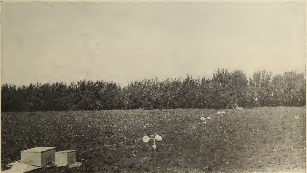
Anemometers placed at various distances away from a shelterbelt indicate a definite reduction in wind velocity for a distance to leeward equal to 20 to 30 tree heights.
