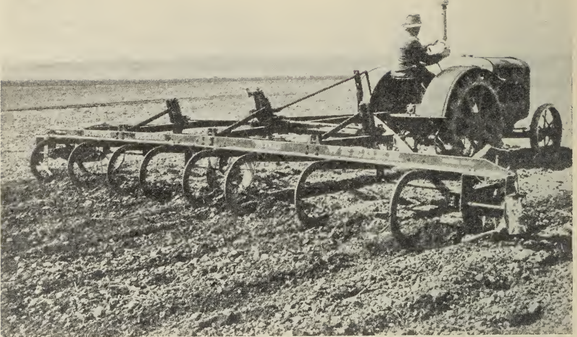
The rod weeder is a very useful implement for destroying weeds on summerfallow land. The soil should first be loosened by the plough or cultivator, the latter implement being used for the final operation for the season. The rod weeder cannot be used in very stony land.
