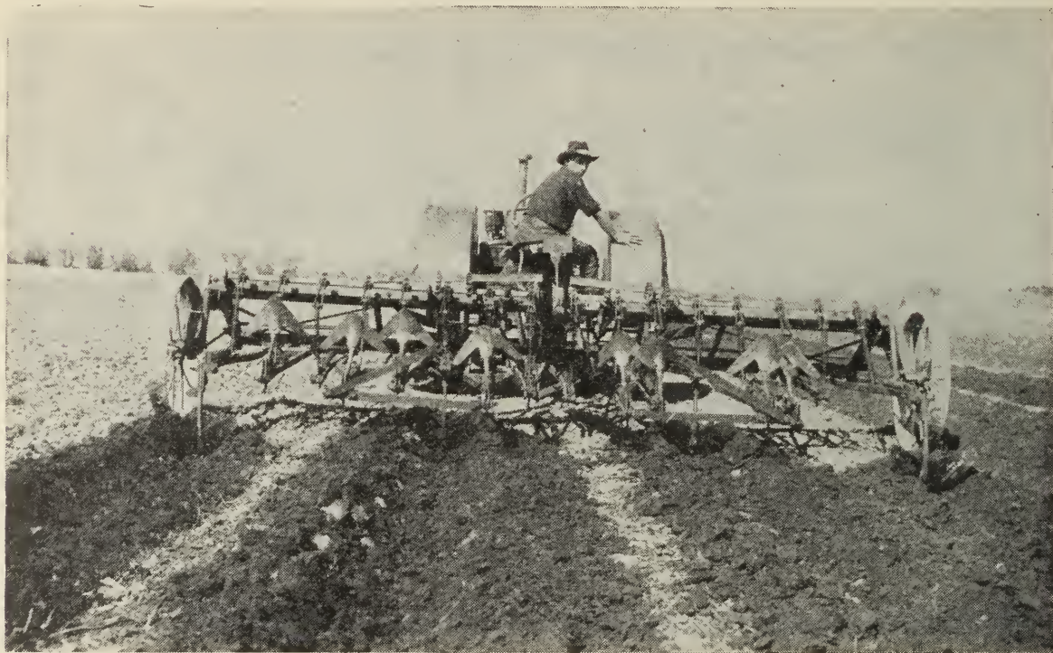
When provided with ridging shovels placed 3 to 4 feet apart, the cultivator is useful for emergency soil drifting control measures. The surface of a field can be quickly transformed into a series of ridges and hollows with this implement.
