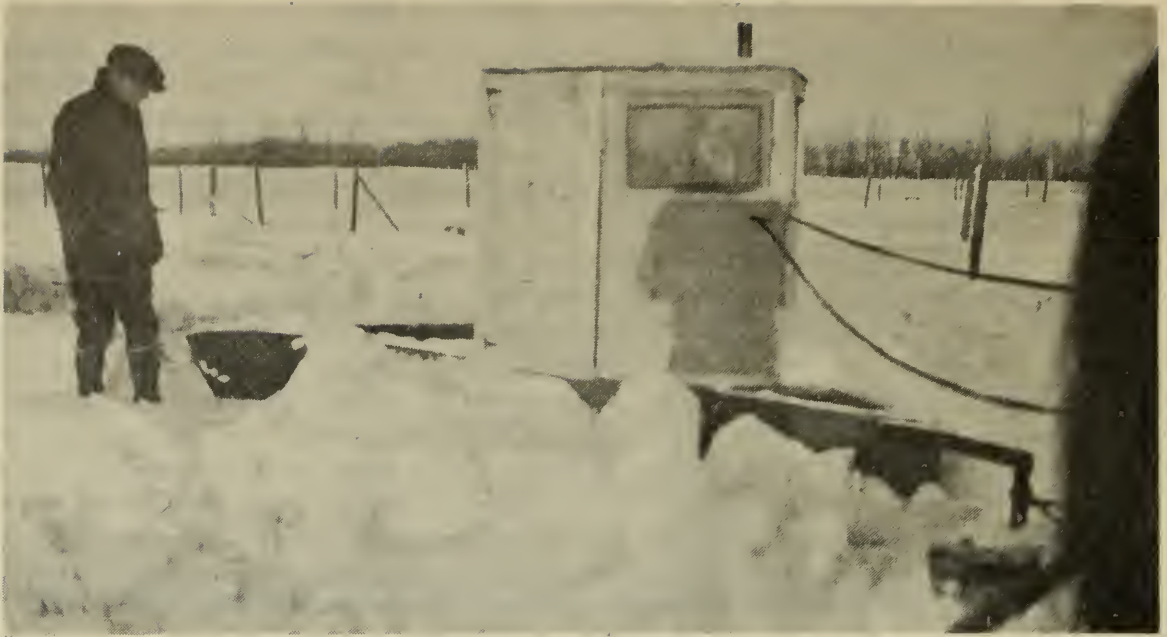
A farmer improved on the pull-type snow-plough by building a cab, with heater, on it. Snow has been removed where the man is standing in order to show a wing attachment designed to throw the ridges higher.
