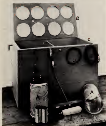
The components needed to build a "Wisconsin temperature tank" for studying root diseases under controlled temperature. (Photograph sent by P.M. Simmonds from the University of Wisconsin to W.P. Fraser, January 9, 1925).
