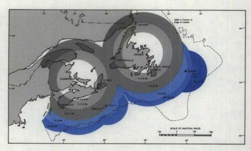
9.6 The Sikorsky S-61 helicopter has an average still-air speed of 115 knots and an endurance time of 5 hours to zero-fuel.
