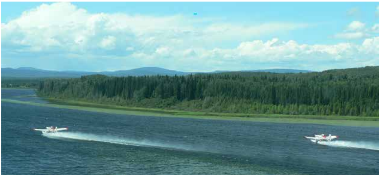
Photo 3. Fire Boss echelon-formation scooping operation
