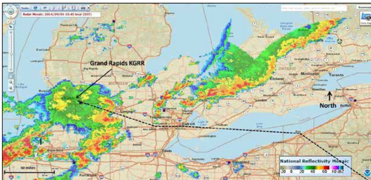
Figure 1. Depiction of weather at time of departure (1845) and the aircraft's planned flight route (dashed line) (Source: National Oceanic and Atmospheric Administration [NOAA], National Weather Service, with TSB annotations)
