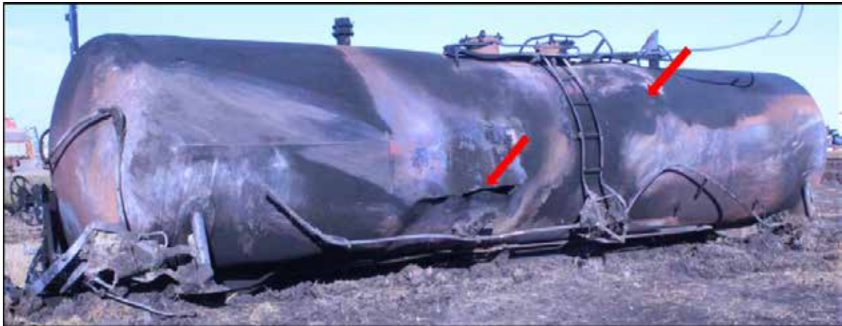
Photo 10. PROX 126 with fire damage and thermal tears (red arrows)
