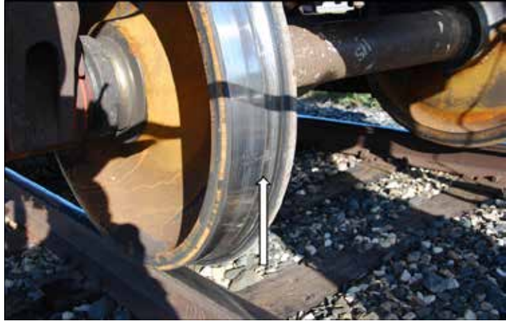
Photo 2. Impact mark on the wheel tread of the trailing wheel of the 31st car (DOWX 3282)
