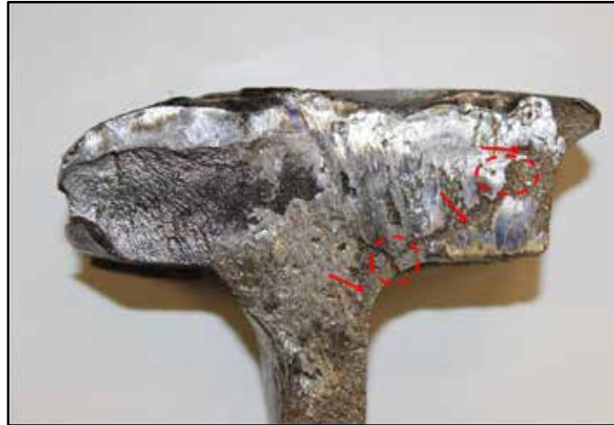
Photo 8. West fracture face of rail piece No. 1 – (Note: Red arrows show the boundary of the detail fracture. Gauge is to the left, field to the right. Red circles indicate areas where fatigue striations were observed.)
