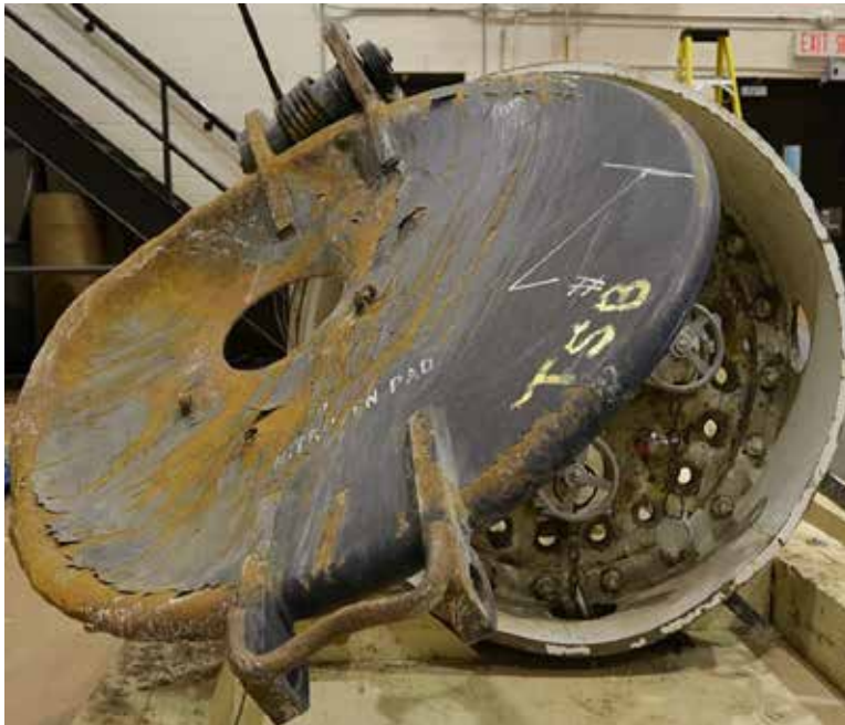
Photo 4. PROX 36178 protective housing and cover
