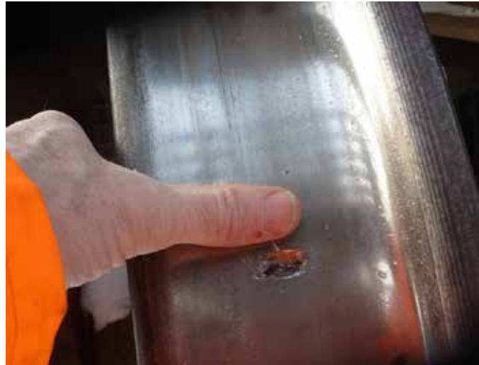
Photo 1. Damaged wheel surface on car PROX 035435
