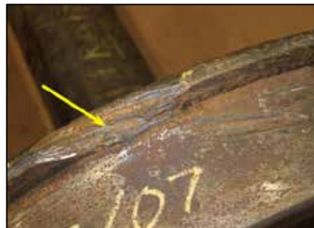
Photo 12. View of mechanical damage on wheel from car DWC 627099
