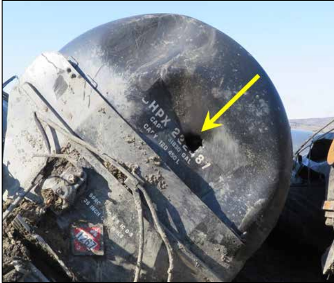
Photo 9. Puncture in unprotected portion of the upper head
