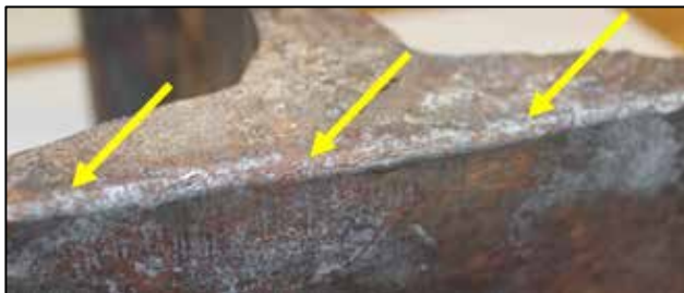
Photo 11. Rounded edge at base of rail piece number 9 (arrows)
