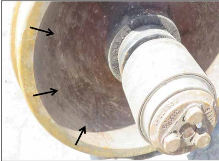
Photo 3. Scuffing on wheel plate, trailing truck of the 61st car (CN 624072)
