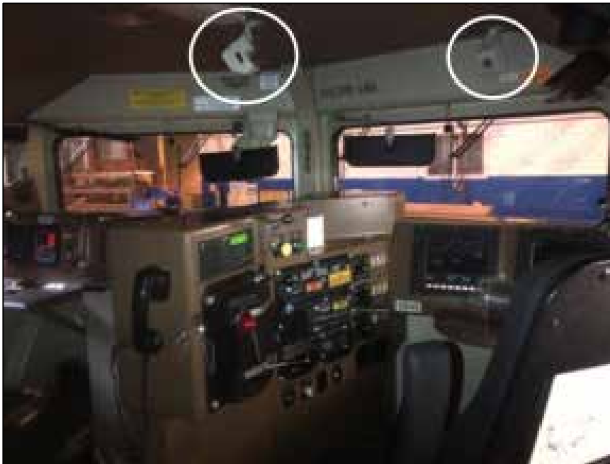
Figure E3. Railway B camera locations on cab ceiling (white circles) (Source: Railway B)
