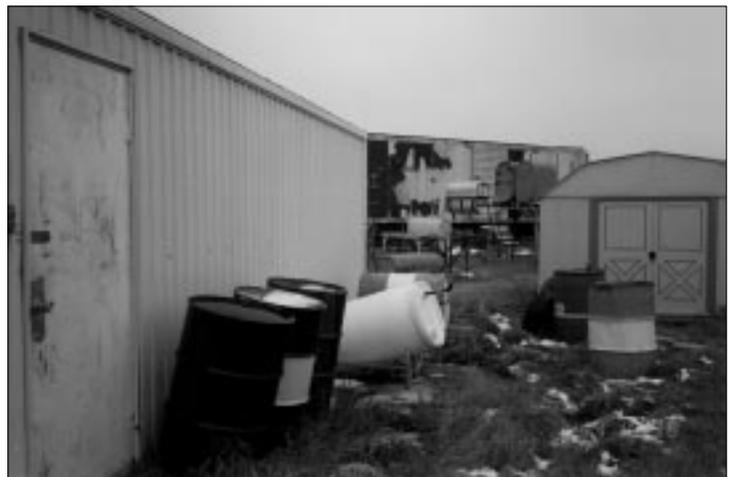
*Drums of oil, solvent and WD10 stored on grass with no secondary containment, alongside a garage at Cold Lake.*
