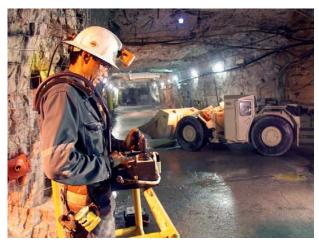
Figure 3: To decrease radiation exposure, a Cameco employee operates a remote-controlled truck to retrieve uranium ore from an underground extraction chamber at the McArthur River mine.
