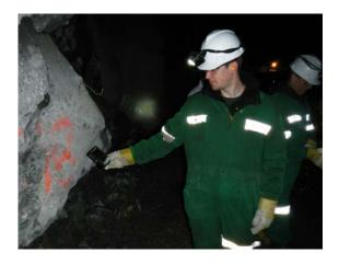
Figure 2: A CNSC inspector takes a gamma radiation measurement at Cameco's Rabbit Lake Eagle Point Mine.
