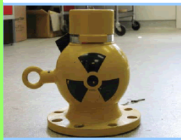
Example of an industrial fixed gauge
