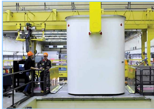
Preparation of used nuclear fuel storage containers
