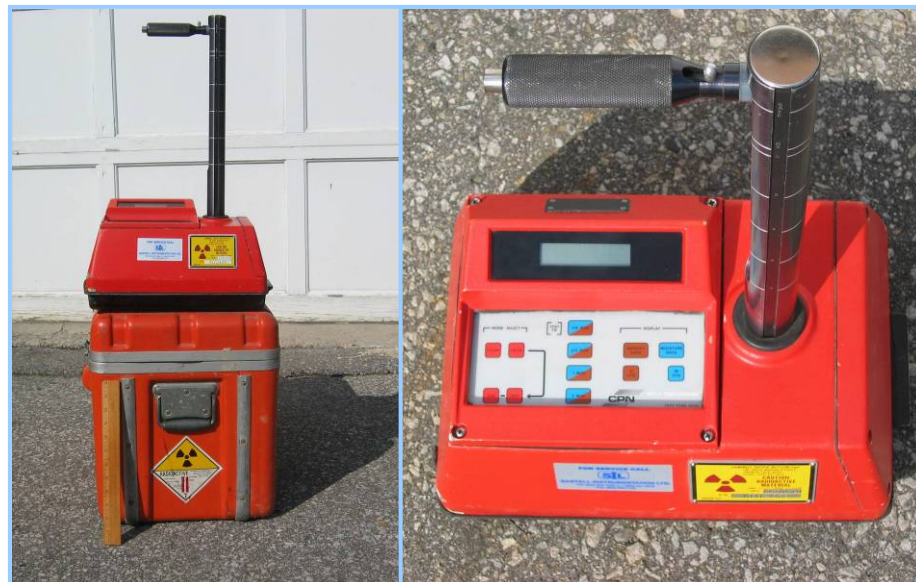
Portable gauge used for paving and geotechnical studies
