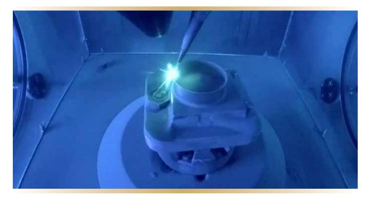
he Fleet Maintenance Facility Cape Scott (FMFCS) laser additive manufacturing (LAM) system was first introduced in the Spring 2014 (No. 73) issue of the *Maritime Engineering Journal*. As explained in the initial article, the system was acquired from the National Research Council (NRC) in London, Ontario.
