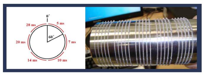
Figure 2. Test Specimen for Parameter Development: The test bar has 25 test strips arranged in five sets of five along the bar. The dial, showing an end-on view of the test bar, illustrates how the pulse duration in milliseconds (ms) was changed at 60-degree intervals around each test strip (for a total of 150 test spots along the bar).
