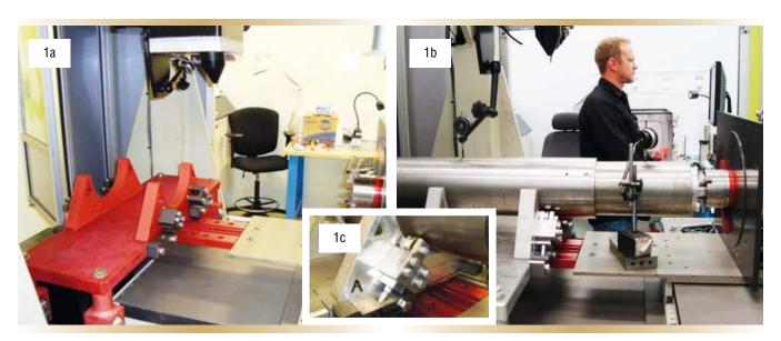
Figure 1a. The shaft LAM jig after application of an anodized protective coating. Figure 1b. The (uncoated) shaft LAM jig with a shaft in-situ to be worked on. Figure 1c. Adjustable rollers permit work to be done on varying shaft diameters.
