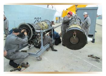
Figure 6. Exchanging connections from the old engine to the new.
