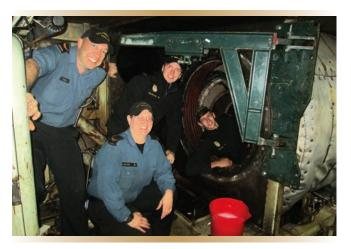
Figure 3. A swivel arm was rigged to manoeuvre the engine in the confined machinery space.
