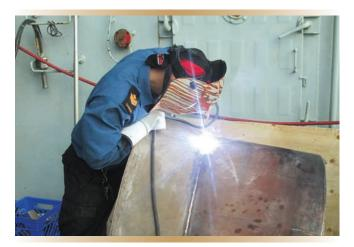
Figure 7. PO2 Boz welds the exhaust diffuser.
