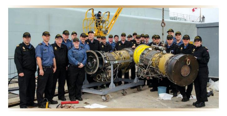
n Sept. 28 2015, while deployed in preparation for exercise Joint Warrior off the west coast of Europe, Her Majesty's Canadian Ship *Athabaskan* (DDG-282) experienced a failure of the starboard cruise gas-turbine engine. This article describes the failure and resultant engine change-out in a foreign port.
