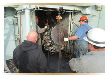
Figure 5. Removing the engine through the bypass doors.
