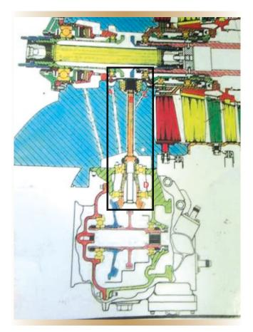
Figure 1. Location of tower shaft between the accessory gearbox and the engine shaft.
