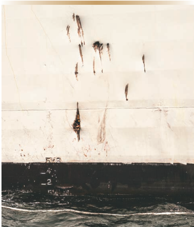
Damage received from the barge outside of the mechanical workshop and forward engine room.
