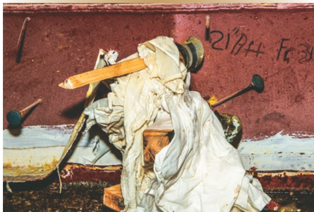
Ship's hull technicians used plugs and wedges to stop the ingress of water while seas were two to three metres high outside the mechanical workshop.
