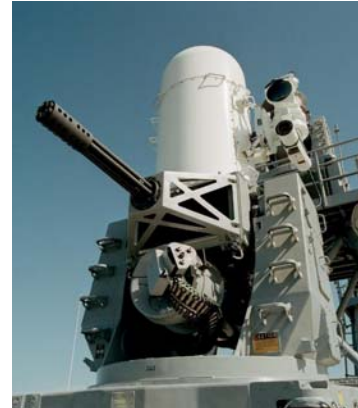
Figure 1. The Close-In Weapon System (CIWS). The CIWS is an anti-missile system mounted on a surface combat ship.
