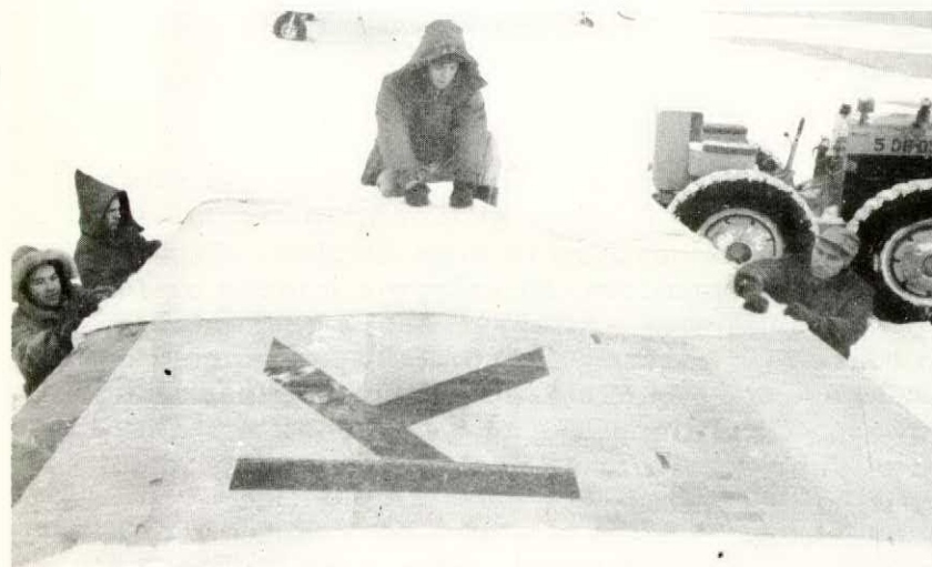
Removing wing covers from a Canuck
