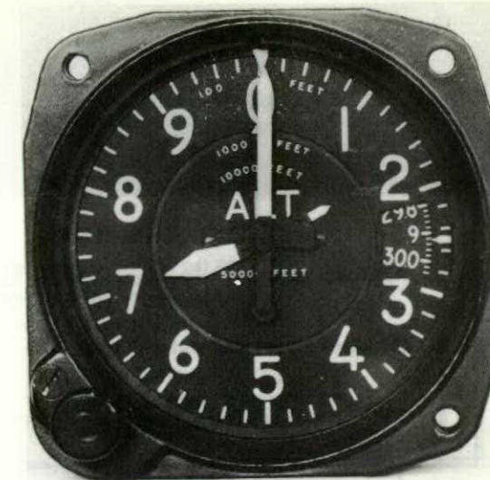
Fig 1. Older model (above) with short pointer, and new model (below) showing long, thin pointer with triangular end.
