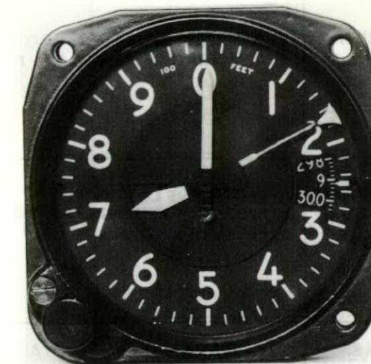
Fig 1. Older model (above) with short pointer, and new model (below) showing long, thin pointer with triangular end.
