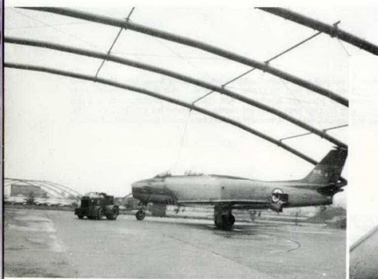
Another overseas Sabre. The towing crew consisted of a driver and a man on the aircraft's brakes. The driver thought he would clear the beam. He didn't—but the disciplinary action taken should assist his thinking in future.
