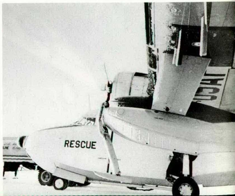
SA16 Albatross of the 54th Search and Rescue Squadron, USAF, at Goose Bay, Labrador, returns from flying the Duck Butt Tango position with load of rime ice.
