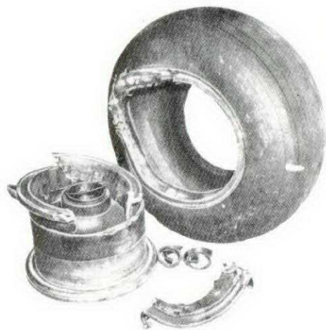
Figure 3 (b) - Landing Gear Wheel and Tire Damaged by Explosion
