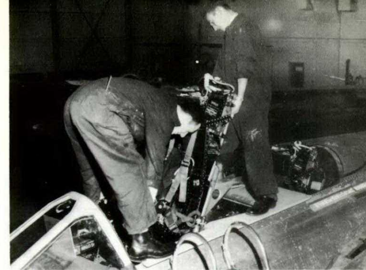
Herewith the Uplands anti-bent canopy rail device. The platform protects both aircraft and personnel.
