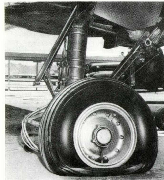
Figure 1 (b) — Left Landing Gear After Outboard Wheel Explosion
