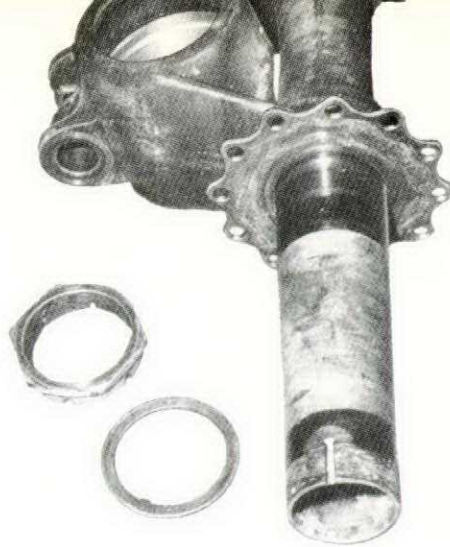
Figure 3 (a) - Landing Gear Axle Assembly Stripped by Exploding Wheel
