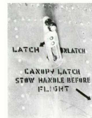
T-33 Canopy External Unlocking Crank Mod. EO 05-50C-6A/158 24 Oct 56
