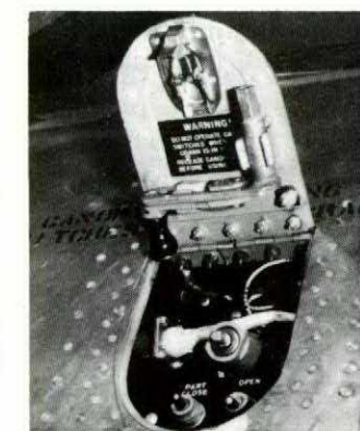
T-33 Canopy External Unlocking Crank Mod. EO 05-50C-6A/158 24 Oct 56
