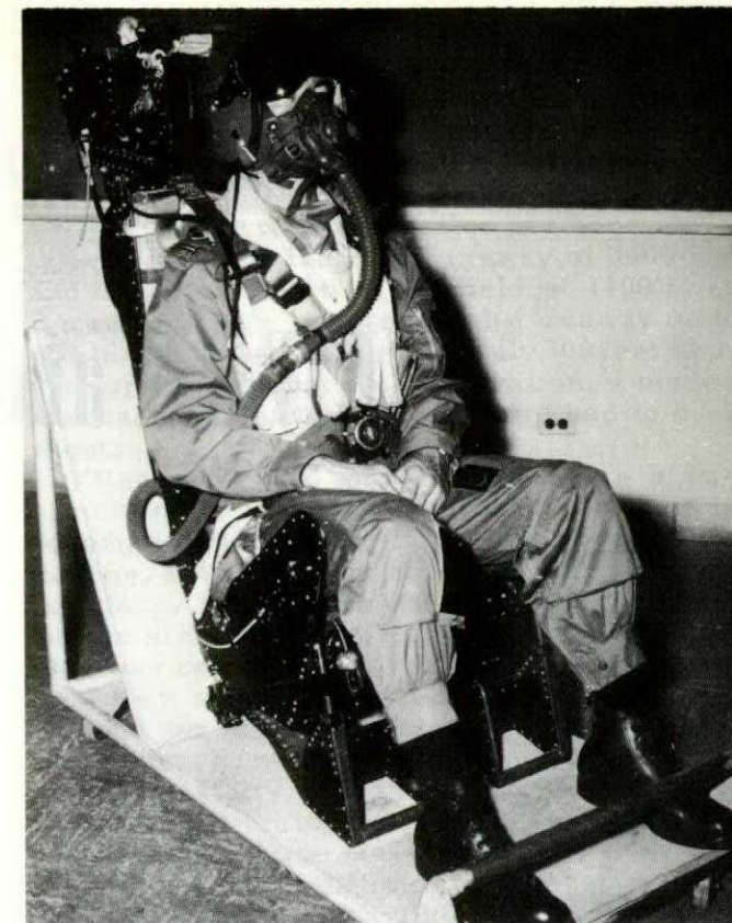
Pictured above is the hook-up arrangement suggested by F/L Thompson. It is obviously the safest and best method. Note that the oxygen line to the bailout bottle has been located behind the lap strap of the safety harness.
