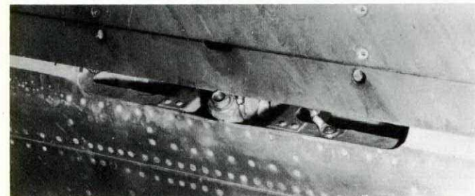
The port aileron actuator piston rod had fractured... jamming the aileron in the "up" position.
