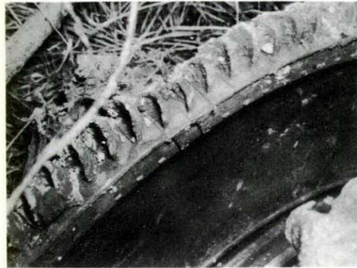
Fig 2. Here is what happens to an overheated turbine blade.
