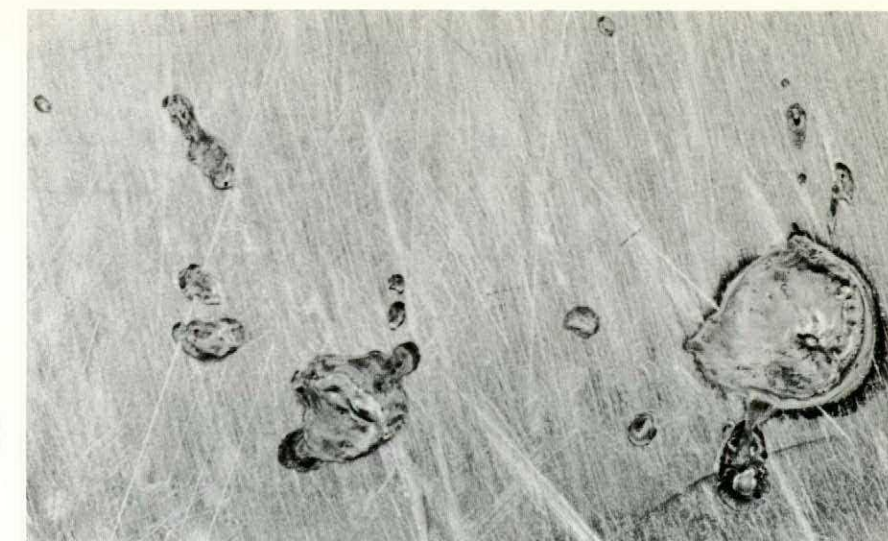
Enlarged view of burn marks on starboard propeller hub.
