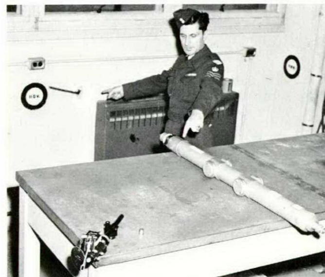
Note dent in drogue gun and damaged wall.
