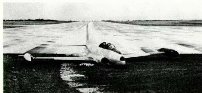
The undercarriage was unserviceable so the aircraft was landed wheels-up on foam.
