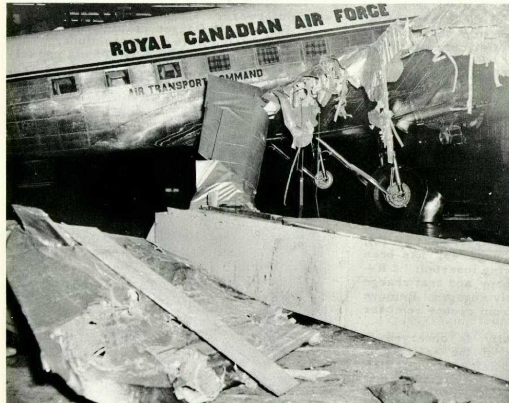
The large rectangular object in the right foreground is the concrete filled counter-weight.
