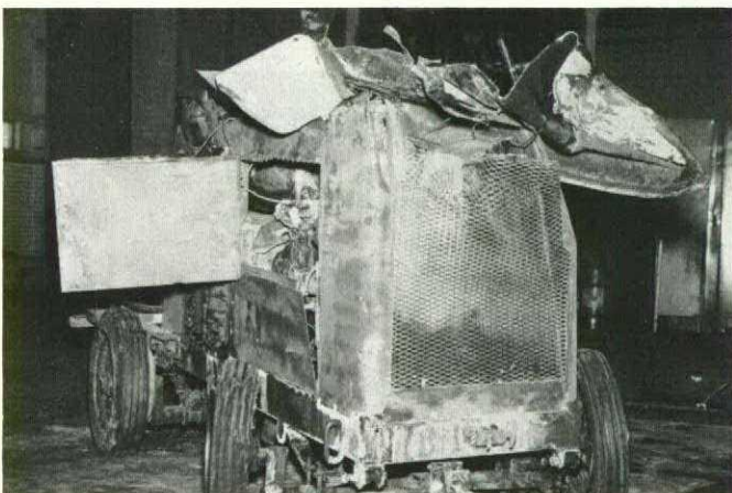
Energizer that was damaged in North Star fire.
