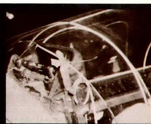
The canopy of a T-33 was closed with the seat arming lever raised.
