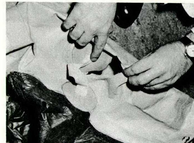
FIG. 4 Ruptured buoyancy chamber of liferaft.
