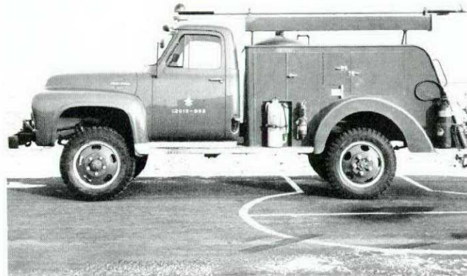
G13 Crash Truck (LRV). The fire fighters "hot-rod". Dual carburetion and dual exhaust give this vehicle rapid acceleration. It carries a complete range of light rescue tools. The long box overhead carries a stretcher, pike pole, and 12-foot folding ladder.
