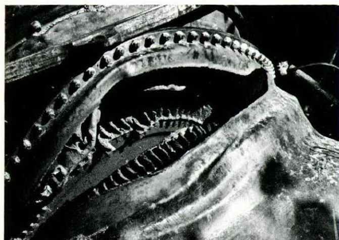
AIB investigators were immediately aware of extreme over temp. Starboard Engine 2nd and 3rd stage turbine wheels illustrate extreme damage from over temp. Port Engine similar emphasizing this happened in a matter of seconds.
