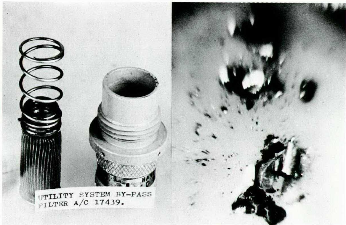
Magnified contamination particles from the steering and shimmy dampening hydraulic system.
