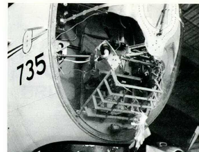
SEAGULL DAMAGE TO NOSE OF ARGUS AIRCRAFT
