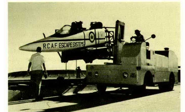
The rocket sled is being lowered onto the breech of the high speed test track at Edwards AFB.
