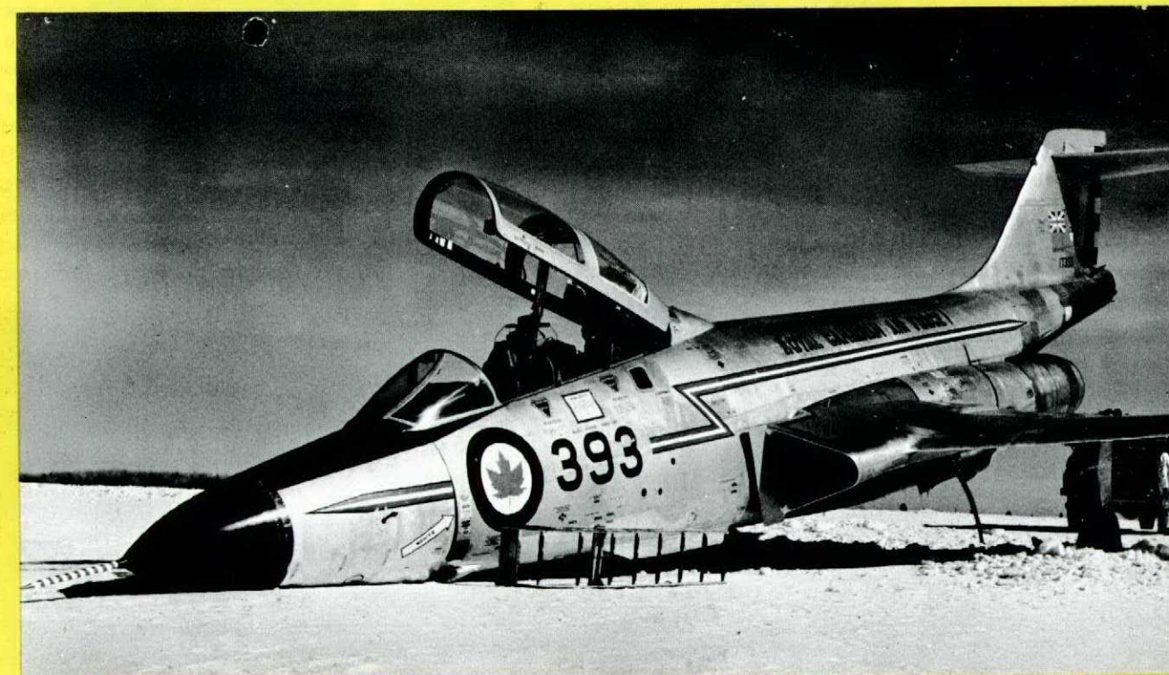
The braking was poor and the barrier failed to function properly—this "runway check" proved both!
