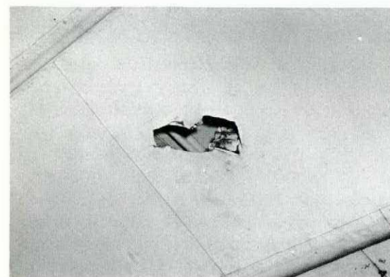
"I wasn't aware of the height of the hydraulic tilt boom on the forklift and I attempted to drive under the port wing."
