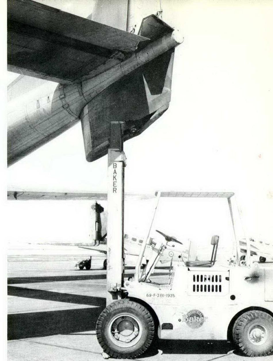
" . . . and I misjudged the height of the boom of the forklift, which struck the tail of the aircraft causing considerable damage."
