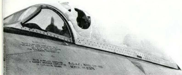
Note how close to the man's head is the front seat break-out area, and how smaller pieces have been punched out
