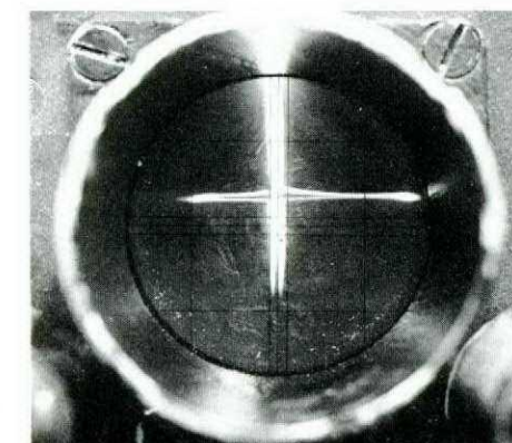
Strong signal showing stronger on right—search aircraft turns to starboard to complete homing
