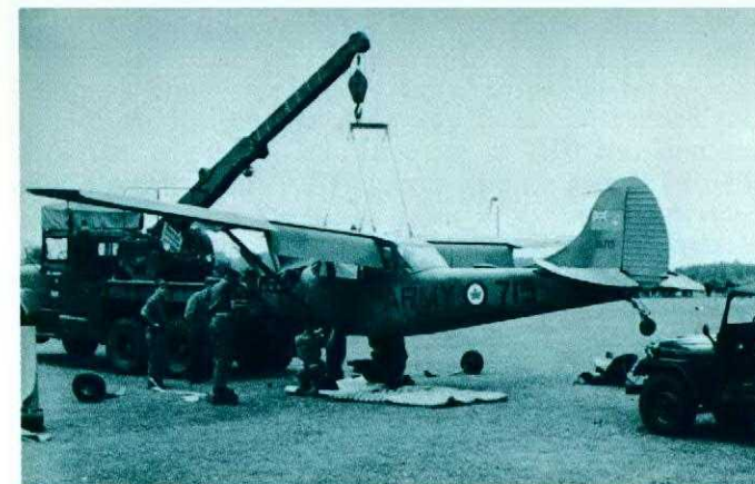
A damaged undercarriage inspected and repaired on an AOP landing ground.
