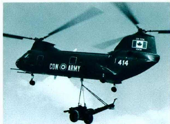
The CH113A cargo helicopters are capable of short haul airlifting 26 troops or up to 8,000 pounds.
