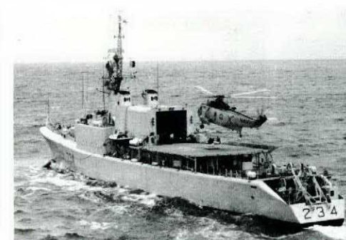
Altitude as aircraft nears deck—positive tension on cable is pulling aircraft down.
