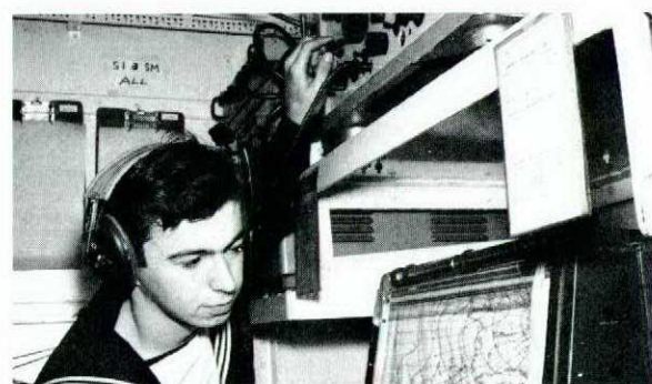
A weather map is received in Bonaventure's meteorological office by radio facsimile
