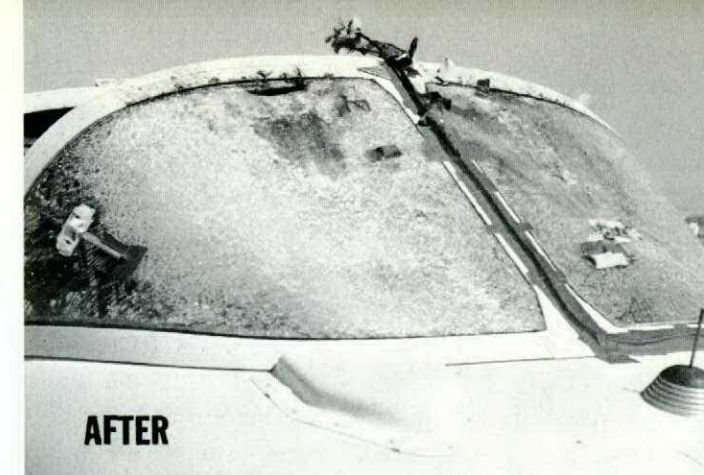
Windscreen damaged by bird strikes
