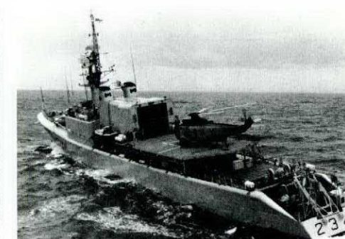
Final touchdown probe is locked in jaws of bear trap.
