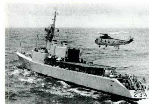
Beginning of landing phase—cable connected to bear trap.
