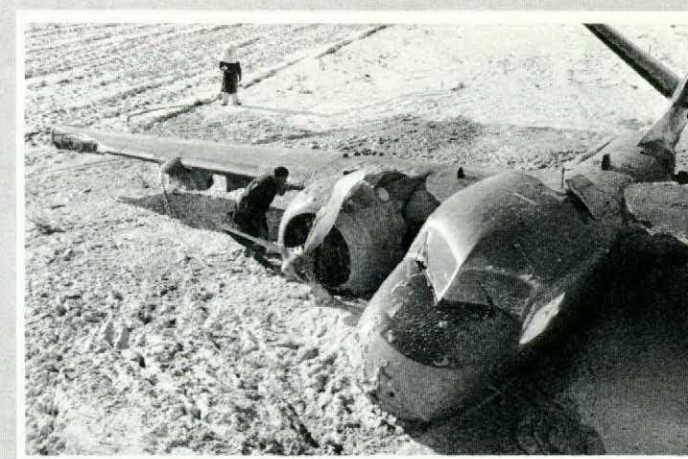
The aircraft had been left out overnight; some wet snow and light freezing rain had frozen to the aircraft. The three pilots on the flight stated they had “looked it over carefully” during their preflight inspection and had chipped most of the ice off. They were sure that the ice remaining would have negligible effect. The captain mentioned somewhat jokingly that he would add ten knots to the takeoff speed just to be sure.
