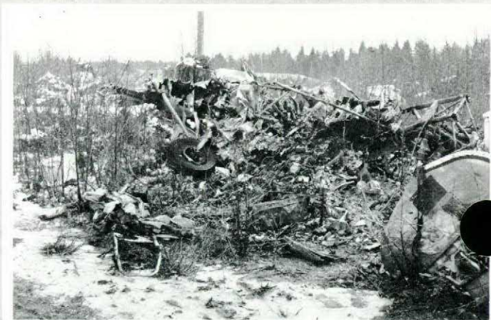
The investigators concluded that the aircraft took off with frost on the wings and crashed right after takeoff.
