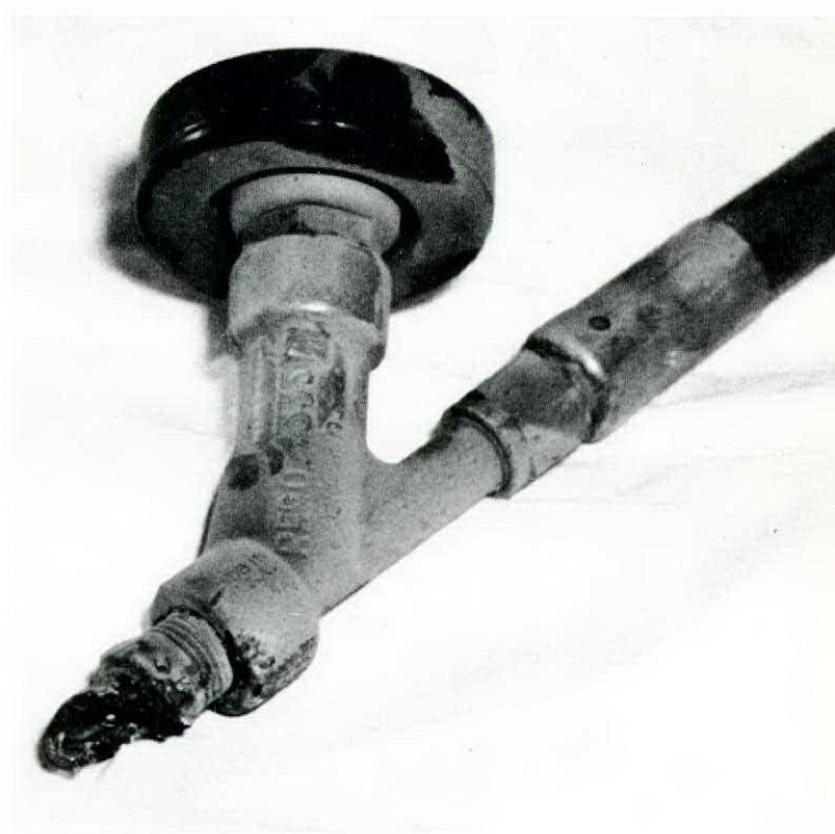
The partially-melted oxygen filler nozzle
