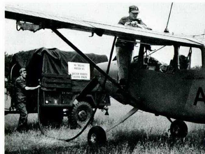
Refuelling from the POL trailer must be done quickly so the aircraft can get under cover as soon as possible.
