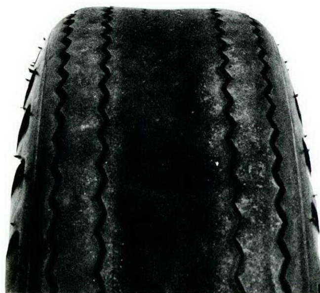
Crown worn from overinflation
